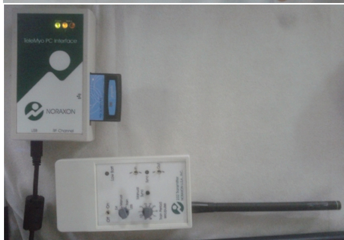
[Table/Fig-2a,b]: a) Telemyo 2400T G2 transmitter with 2 or 3-snap EMG lead connected and Inline wireless Sync Receiver connected; b) Telemyo 2440T G2 PC interface connected to USB cable.
